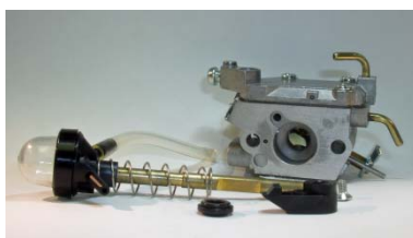
4. Assemble new Primer kit with original spring and plastic ring
