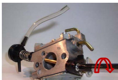
5. Re-assemble original lever and screw
