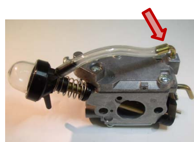
6. Connect hose onto brass fitting
