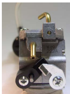
5. Re-assemble original lever and screw
