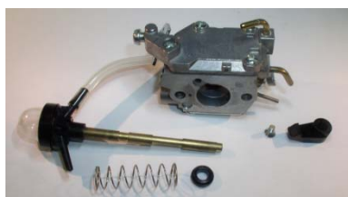
4. Assemble new Primer kit with original spring and plastic ring
